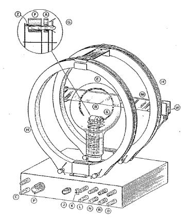
Figure 2.1: Charge-to-Mass Ratio Apparatus.
